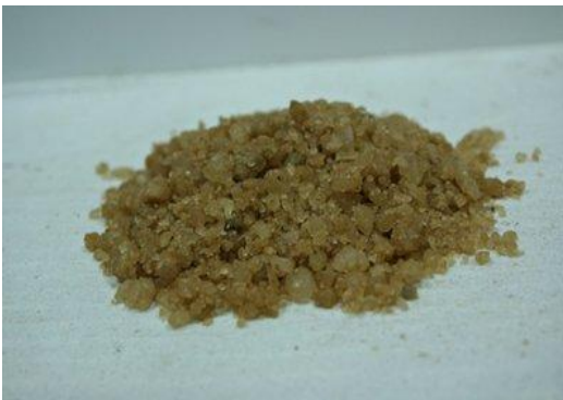
Salt treated with Beet Heet (pictured here) melts 65% more ice than untreated rock salt in an hour at 25°F, the company said. Photograph: K-Tech Specialty Coatings
