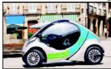
MINI ME: The 8ft-long Hiriko Fold shrinks down to 5ft when it's parked
