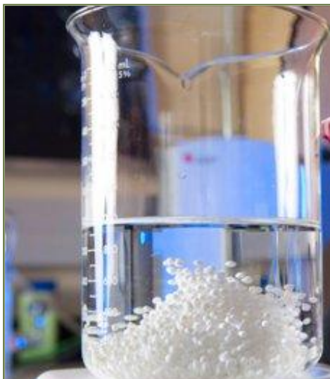
Zimmerman Lab developed chitosan beads impregnated with titanium dioxide and aluminum oxide. These beads are used for the removal of heavy toxic metals, like arsenic and selenium, from water. (Photo Credit: Harold Shapiro)
